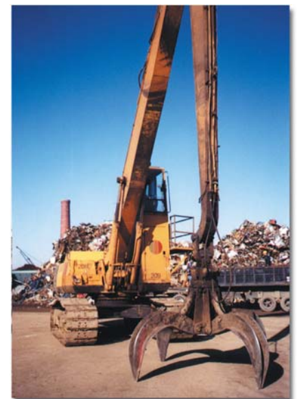
Komatsu PC 400 with 32" wide TUFPADS Track Pads, used in steel recycling yard
