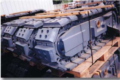
Track assemblies with TUFPADS® , awaiting installation on new milling machines
