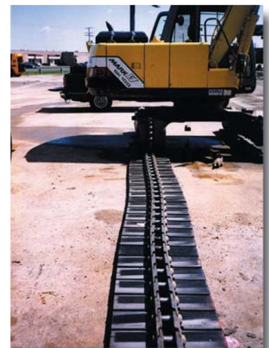
Track Chain with TUFPADS® attached, ready to install on Kobelco SK 100 Mark IV
