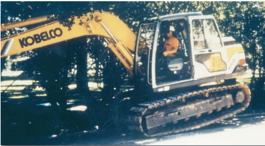
Kobelco SK 120 backhoe using TUFFPADS ® track pads on an asphalt surface
