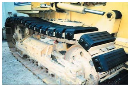
Artliner-BLS Clip-On Track Pads with bolts
