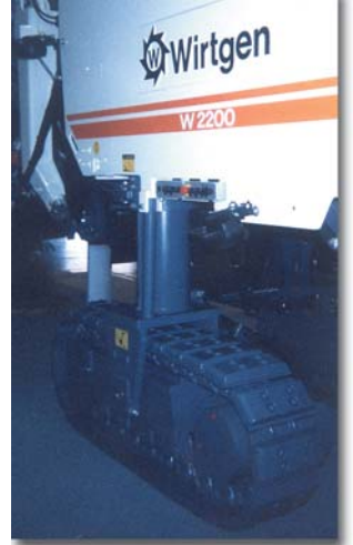
Newest model milling machine from Wirtgen, the W2200, using TUFPADS® track pads
