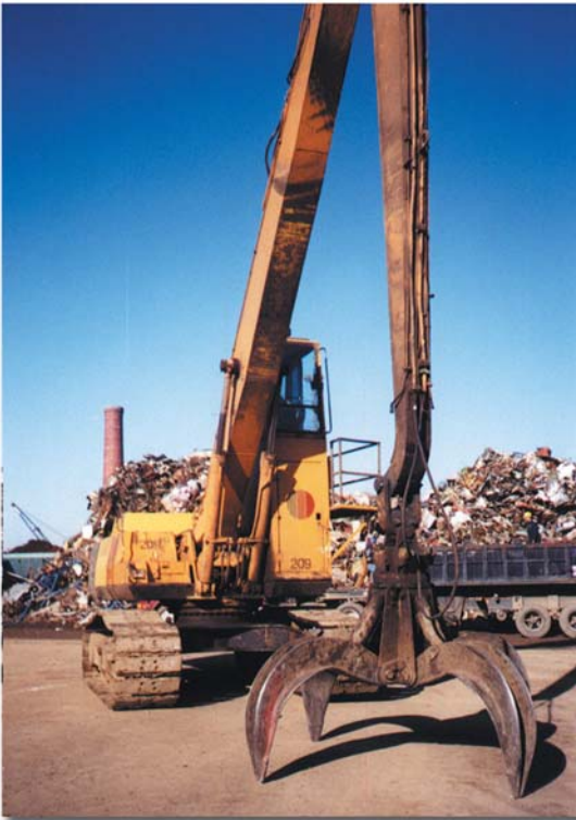
Komatsu PC 400 with 32" TUFPADS ® in steel recycling yard. These pads eventually wore out after more than 2000 hours of very abusive duty.
