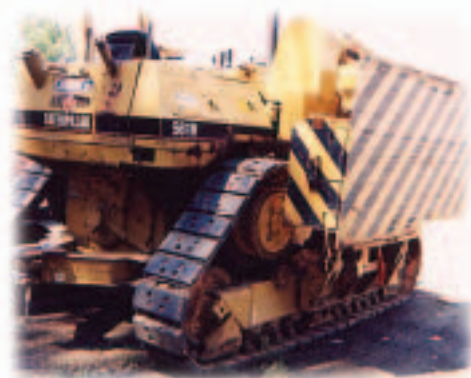
TUFPADS® on Caterpillar 561H Cable Layer
