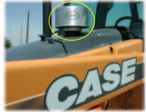
CENTRI® Air Precleaner on Case 580 Backhoe
