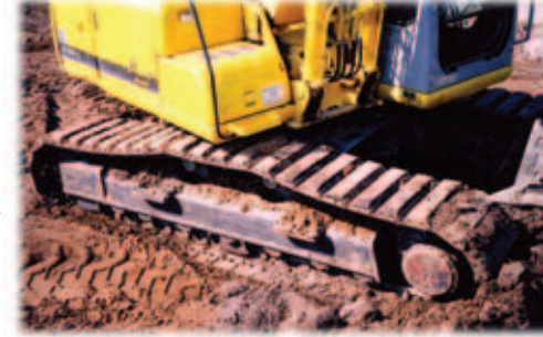
Artliner-BLS Track Pads on Kobelco SK160LC
