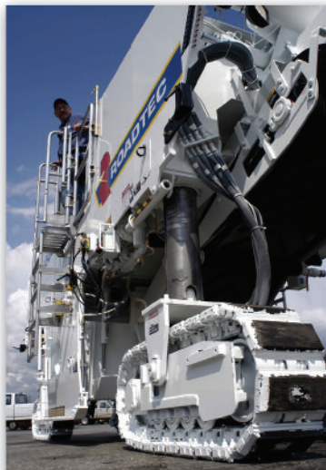
BLS Poly Bolt-On® Track Pads on a Roadtec RX-500 milling machine
