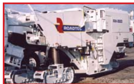
BLS Poly Bolt-On ® Track Pads on a Roadtec RX-900 milling machine
