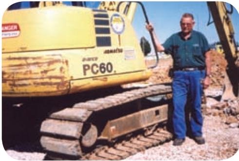
3,694 hours on the Artliner-BLS rubber treaded on Jim Geedings Komatsu PC-60
